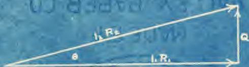
Fig. 8. Vector Relations in Method of Measuring Ratio and Phase Angle.
